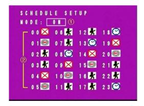
① SCHEDULE SETUP : Record ON / OFF setup (default setup is OFF).
